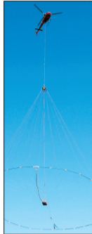
A helicopter (left) lowers the time-domain electromagnetic (TEM) geophysical system into position
